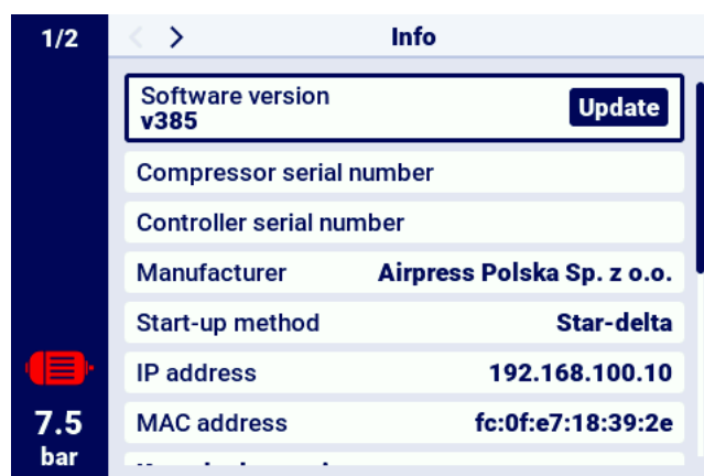
Figure 49: The "Information" tab with the IP and MAC address.
