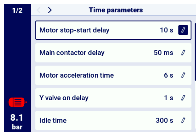
Figure 25: View of the menu with time parameter settings for the Star-Delta configuration
